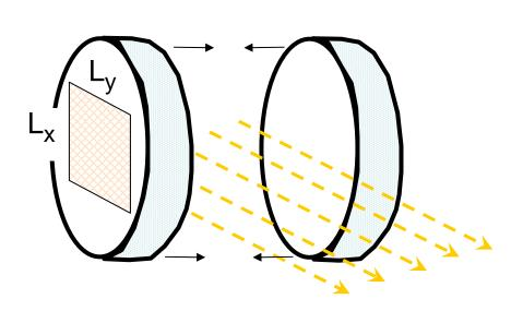
Probe beam parallel to the plane of the condensates
