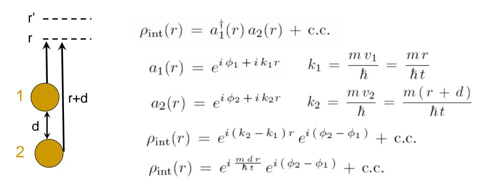
Clouds 1 and 2 do not have a well defined phase difference. However each individual measurement shows an interference pattern
